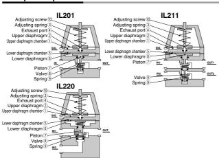
The signal air pressure enters the upper diaphragm chamber ① to generate a force. When this force is larger than the force generated by compressing the adjusting spring ③, the upper diaphragm ② is pushed up, the exhaust port ④ is closed, and the signal air pressure enters the lower diaphragm ⓒ. This pushed down the piston ⑦ to open the valve.
