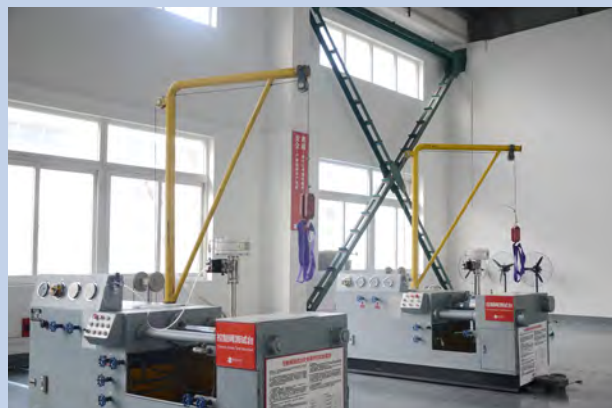
© 源冠自控控制阀性能测试台 © control valve test machine of champion controls
