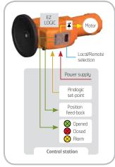
EZ LOGIC integrated control Positioning version
