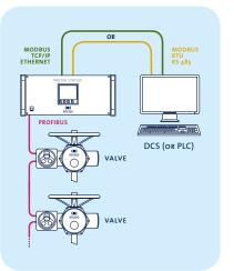
MS101 – The simple fieldbus solution. One 19" rack to set up, control and command your network of actuators. A single MS, a single line, up to 3 starts of lines.
