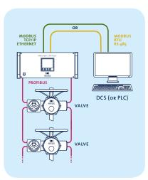
MS102 – Line redundancy for improved reliability. One 19" rack plus a second cable for line redundancy: more security in case of default of one cable. A single MS, a redundant line, up to 3 starts of lines.
