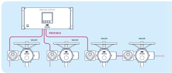
Fieldbus is interesting because it allows getting more information while reducing the overall cost of wiring and commissioning on site. Our Master Station goes further and optimizes the cable length needed to connect your actuators thanks to the **possibility to have 1 to 3 different starts of lines**. Such advantage is especially appreciated if you have 2 or 3 groups of actuators located in opposite directions, and makes you save time and resources.
