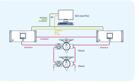
MS202 – System and Line redundancy. Two 19" racks featuring line redundancy. In this configuration, if the first unit is out of service, the second one ensures proper communication with the entire network. Two MS, a redundant line, up to 3 starts of lines.
