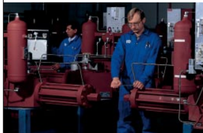
Gas/oil actuators undergoing final inspection before shipping
